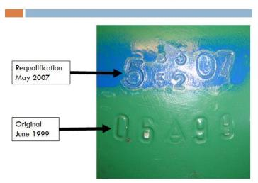
The above cylinder was originally tested in June 1999 and was requalified in May 2007. The picture below shows the tank would expire on May 2012. The cylinder does not have a star  $(\mbox{$^{\upsym}$})$  which would indicate it would not expire for 10 years from the date of the stamp. The tank should be removed from service until requalification of hydrostatic testing is completed once it expired.
